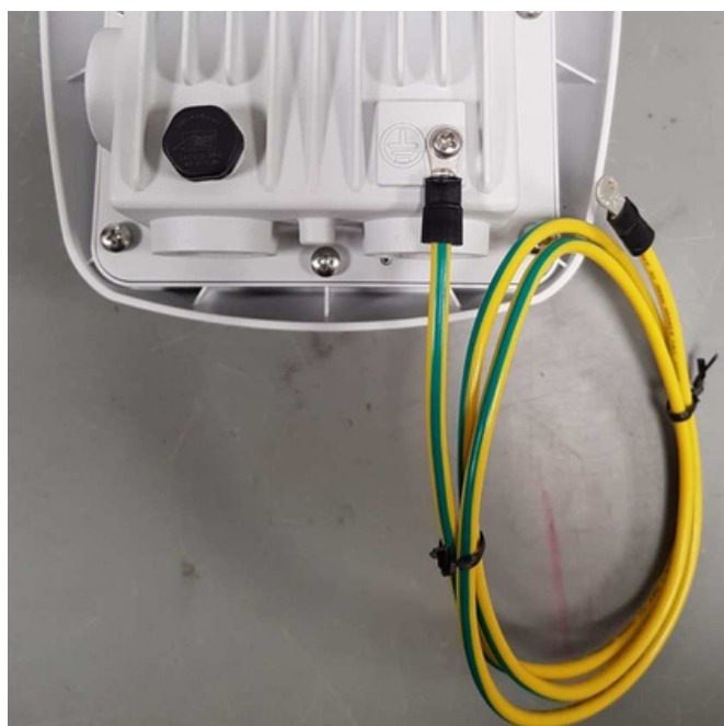
Figure 12: Earthing with mounting kit provided
