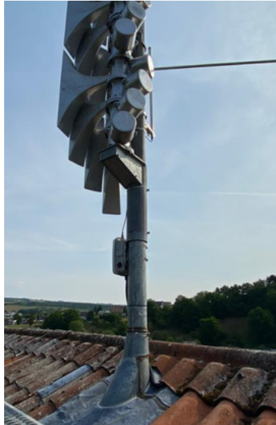
LoRaWAN-Gateway (8 Kanal) (Fa. Kerlink, Wirnet iStation)
